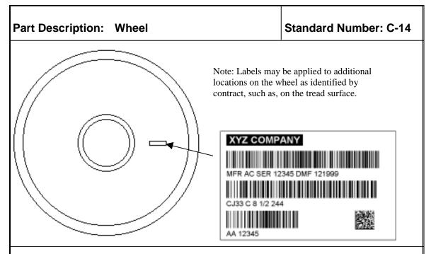
**Label Description**: A two-part durable label will be affixed to the serialized component. It will show the OEM Equipment Manufacturer Number, Serial Number and Manufacture Date on one section. The second section will show the Wheel Design, Wheel Class, Bore Size, AAR Tape Size, and Heat Number. The label material will be weather resistant and use permanent adhesive. Information will be machine and human readable.
