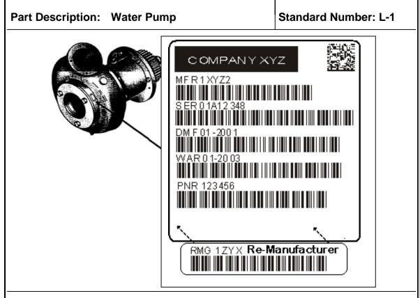
**Label Location:** Label shall be affixed or applied in a way that does not interfere with the operation of the component; in a conspicuous location to facilitate ease of reference while in service, disassembled and while in transport. Suggested location for label is indicated above.
