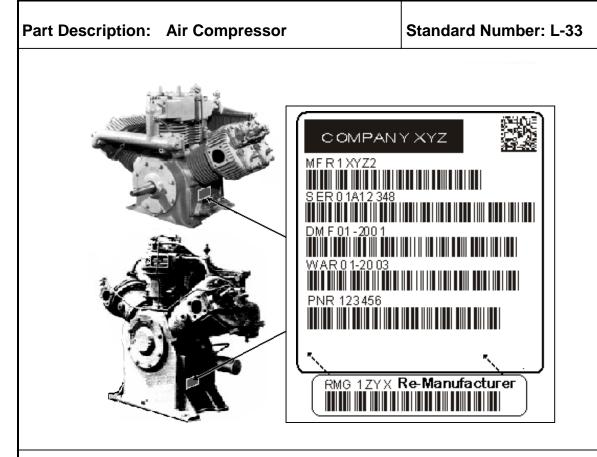
**Label Location:** Label shall be affixed or applied in a way that does not interfere with the operation of the component; in a conspicuous location to facilitate ease of reference while in service, disassembled and while in transport. Suggested location for label is indicated above.
