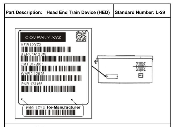
**Label Location:** Label shall be affixed or applied in a way that does not interfere with the operation of the component; in a conspicuous location to facilitate ease of reference while in service, disassembled and while in transport. Suggested location for label is indicated above.
